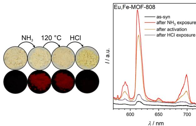
**Fig. 6** Color changes based on ligand exchange and fluorescence switching recorded under UV light (254 nm, left) and fluorescence spectra of as-synthesized Eu,Fe-MOF-808 ( $\lambda_{\text{ex}} = 296$  nm, right) before and after all steps of the read-out sequence measured under ambient conditions.
