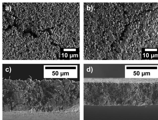
**Fig. 9** Top view SEM images of (a) Co- and (b) Fe-MOF-808@PVDF, as well as cross-section SEM images of (c) Co- and (d) Fe-MOF-808@PVDF.
