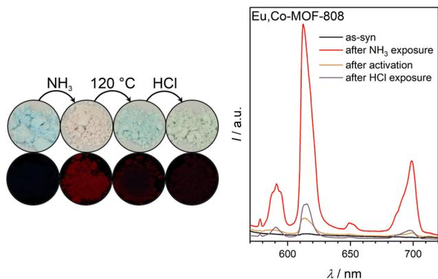
**Fig. 5** Color changes based on ligand exchange and fluorescence switching recorded under UV light (254 nm, left) and fluorescence spectra of as-synthesized Eu,Co-MOF-808 ( $\lambda_{\text{ex}} = 296$  nm, right) before and after all steps of the read-out sequence measured under ambient conditions.
