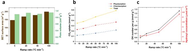
Fig. 1 (a) BET surface area and pore volume for 400-2 h-X samples, (b) CO<sub>2</sub> adsorption for 400-2 h-X samples at 40 °C and 100 kPa and (c) surface hydroxyl numbers for 400-2 h-X samples.
