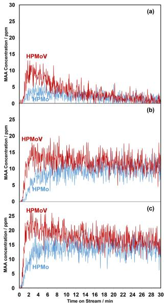
Fig. 1 Comparison of the evolution of MAA formation at 320 °C as a function of time on stream over H<sub>3</sub>PMoO<sub>12</sub>O<sub>40</sub> and H<sub>4</sub>PMoO<sub>11</sub>VO<sub>40</sub> under MAL (a), MAL +  $O_2$  (b), and MAL +  $O_2$  +  $H_2O$  (c). The gas feed is composed of 3500 ppm MAL (when added), 7000 ppm O<sub>2</sub> (when added), 7000 ppm H<sub>2</sub>O (when added), and Ar balance and the total flow rate is 100 cm<sup>3</sup> min<sup>-1</sup>.
