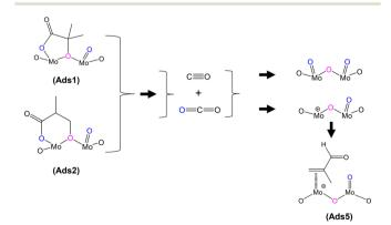
Fig. 5 Proposed formation of by-products CO and  $CO_2$  derived from lactone-type adsorbed species during MAL adsorption at 320 °C.
