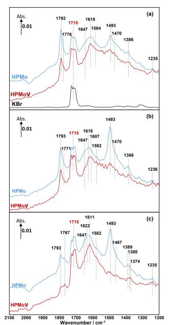
Fig. 2 Comparison of *in situ* DRIFT spectra recorded at 320 °C over  $H_3PMoO_{12}O_{40}$  and  $H_4PMoO_{11}VO_{40}$  at 2 min under MAL (a), MAL +  $O_2$  (b), and MAL +  $O_2$  +  $H_2O$  (c). The gas feed is composed of 3500 ppm MAL (when added), 7000 ppm  $O_2$  (when added), 7000 ppm  $H_2O$  (when added), and Ar balance and the total flow rate is 100 cm<sup>3</sup> min<sup>-1</sup>.
