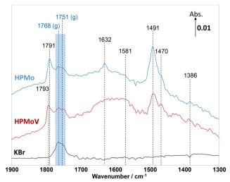
Fig. 4 Comparison of *in situ* DRIFT spectra recorded at 2 min during the adsorption of methacrylic acid (MAA) at 320  $^{\circ}$ C over  $H_3$ PMoO<sub>12</sub>O<sub>40</sub> (HPMo),  $H_4$ PMoO<sub>11</sub>VO<sub>40</sub> (HPMoV), The gas feed is composed of 3500 ppm MAA and Ar balance and the total flow rate is 100 cm<sup>3</sup> min<sup>-1</sup>.
