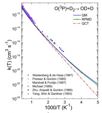
Fig. 8 Same as Fig. 7 for the  $O(^3P) + D_2$  reaction. Experimental results: Westenberg and de Haas, <sup>8</sup> Presser and Gordon, <sup>13</sup> Marshall and Fontijn, <sup>15</sup> Michael, <sup>23</sup> Zhu et al. <sup>24</sup> and Yang et al. <sup>19</sup>
