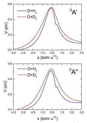
Fig. 1 Vibrationally adiabatic minimum energy paths for  $O(^{3}P) + H_{2}$  (blue) and  $O(^{3}P) + D_{2}$  (red) reactions as a function of the mass-scaled reaction coordinate (see text for definition) on the 3A' (upper panel) and 3A" (bottom panel) PESs calculated by Zanchet et al.<sup>27</sup> In both cases, the minimum energy paths for the two isotopes are referred to as the respective ZPE of H<sub>2</sub> and D<sub>2</sub>
