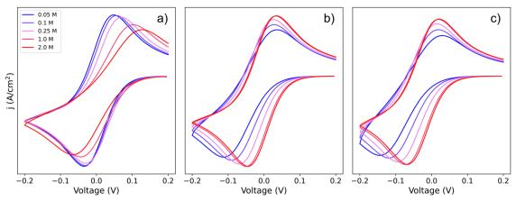
Fig. 2 Simulated cyclic voltammograms for each of the pathways depicted in Scheme 2: pathways, (a) 1, (b) 2, and (c) c. The three plots are computed using  $K_A^Q = 2$ ,  $K_A^R = 10$  and  $k_1^0 = k_2^0 = k_3^0 = 0.01$ , all with a scan rate of 50 mV s<sup>-1</sup> and [Q] = 5 mM, for [Li<sup>+</sup>] ranging from 0.05–2 M.
