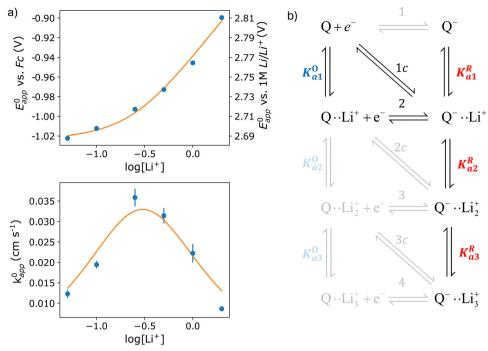
Fig. 4 (a) Experimental standard potential,  $E^0$  (top) and kinetic constant,  $k^0$  (bottom) represented as dots compared with the fitting results when assuming the mechanism represented in panel (b). The values derived from the fits are given in Table 1. (b) Schematic of the possible pathways for redox activity of DBBQ in Li<sup>+</sup> containing DMSO solutions. The greyed-out pathways were not needed to explain the experimental behaviour.
