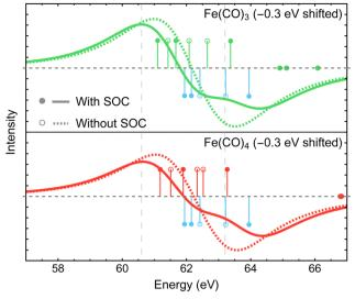
Fig. 7 Difference Fe 3p X-ray photoelectron spectra of Fe(CO)<sub>3</sub> and Fe(CO)<sub>4</sub> relative to Fe(CO)<sub>5</sub> simulated using MR-ADC(2)-X with and without spin-orbit coupling (SOC) effects. Vertical lines represent the computed core ionization energies and the corresponding photoelectron intensities. Blue lines correspond to Fe(CO)<sub>5</sub>. See Section 3 for computational details
