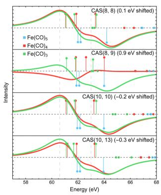
Fig. 8 Difference Fe 3p X-ray photoelectron spectra of  $Fe(CO)_3$  and Fe(CO)<sub>4</sub> relative to Fe(CO)<sub>5</sub> simulated using MR-ADC(2)-X with different selections of active space orbitals in the reference CASSCF calculations. Vertical lines represent the computed core ionization energies and the corresponding photoelectron intensities. Blue lines correspond to Fe(CO)<sub>5</sub>. See Section 3 for computational details.
