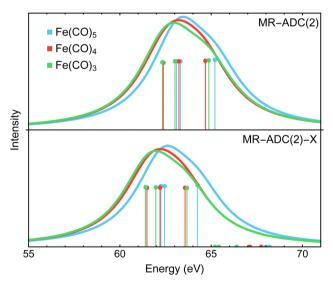
Fig. 4 Fe 3p X-ray photoelectron spectra of Fe(CO)<sub>5</sub>, Fe(CO)<sub>4</sub>, and Fe(CO)<sub>3</sub> simulated using MR-ADC(2) and MR-ADC(2)-X. Vertical lines represent the computed core ionization energies and the corresponding photoelectron intensities. Calculations employed the CAS(10e,13o) active space and uncontracted def2-TZVPP basis set. See Section 3 for more computational details
