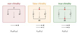
Fig. 7 Barron's classes of chirality and their examples. The systems M and  $M^*$  are mirror images of each other. In all cases,  $\sigma$  denotes a mirror plane,  $\hat{R}$ a proper rotation, and  $\hat{\theta}$  the time-reversal operation. The magnetic field **B** is an axial time-odd vector, the electric field  $oldsymbol{\mathcal{E}}$  is a polar time-even vector, and the propagation k is a polar time-odd vector.
