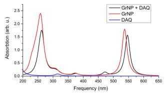
Fig. 8 Theoretical UV absorption spectra of the graphene-DAQ binary complex computed at TDDFT/\omegaB97X-D3BJ/def2-TZVPP level of theory.
