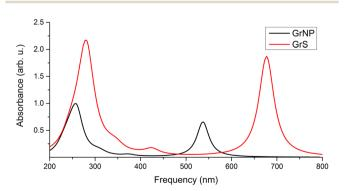
Fig. 4 Theoretical UV absorption spectra of the model graphene lattice both in the optimized (GrNP) and fixed (GrS) geometry forms, computed at TDDFT/ωB97X-D3BJ/def2-TZVPP level of theory.
