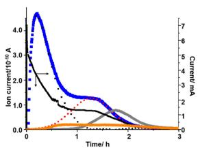
Fig. 6 Time dependencies of current (black) and signals of m/z = 18(orange), 32 (blue), and 44 (gray) when the voltage was stepped from 2.8 V to 4.4 V. The red dotted line shows Gaussian fitting for the 2nd oxygen generation and the black dotted line is the residue for O2 generation after the subtraction of the red curve.
