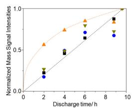
Fig. 8 Discharge time dependencies of integrated signal intensities, i.e., current ( $\nabla$ ), and ion current of m/z = 18 ( $\triangle$ ), 32 ( $\bullet$ ), and 44 ( $\blacksquare$ ), normalized by those of 9.6 h discharge.
