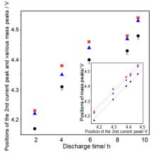
Fig. 9 Positions of the second peak of current (+), 18 (■), and 32 (●), and the peak of 44 (A) as a function of discharge time. Inset: Positions of the second peak of 18 (■) and 32 (●), and the peak of 44 (△) as a function of the positions of the second current peak.
