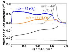
Fig. 2 Typical discharge/charge curves (bottom panel) and ion currents of the Q-mass at m/z = 18 (H<sub>2</sub>O), 32 (O<sub>2</sub>), and 44 (CO<sub>2</sub>) during charge (top panel) of a Li/TEGDME-1M LiTFSI/KJCNT cell (electrode area: 2 cm<sup>2</sup>) obtained under a constant current of 0.4 mA (0.2 mA cm $^{-2}$ ).
