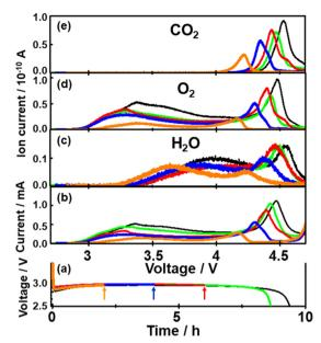
(a) Discharge curves of various cells with discharge times of 2 (orange), 4 (blue), 6 (red), 8.8 (green), and 9.6 h (black). (b)-(e) Potential dependencies of (b) current and the background corrected ion currents of mass signals of (c) m/z = 18 (H<sub>2</sub>O), (d) 32 (O<sub>2</sub>), and (e) 44 (CO<sub>2</sub>) as a function of time for 2 (orange), 4 (blue), 6 (red), 8.8 (green) and 9.6 h (black) discharged cells.
