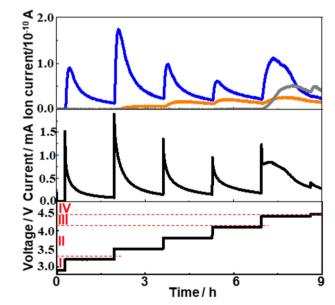
Fig. 5 Time dependencies of current (middle panel) and mass signal of m/z = 18 (orange), 32 (blue), and 44 (gray) (top panel) when the sequences of the voltage step (300 mV step and 6000 s stay before the next step) were applied as shown in the bottom panel.
