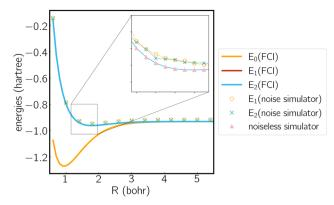
Fig. 1 Potential energy curve calculated by FCI as well as noiseless and noise simulators. Molecule is treated in the  $D_{3h}$  symmetry, where the polar coordinates of the three hydrogen atoms are (R,0),  $(R,\pi)$  and  $(\sqrt{3}R,\pi/2)$ . Note that E<sub>1</sub> and E<sub>2</sub> are degenerate in FCI result due to symmetry.
