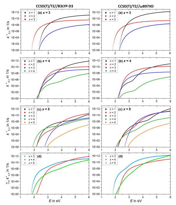
Fig. 8 (a)–(c) Calculated RRKM rate constants  $k_{x,n}^+$  for the loss channels (2) of the precursor ions (NaCl)<sub>x</sub>Na<sup>+</sup> with x = 3-5. Note that the loss channels producing Na<sup>+</sup> ions ( $k_{x,n=x}^+$ ), which cannot be detected in the experiment, are always the slowest at higher energies. (d) Total fragmentation rate constants  $\sum k_{x,n}^+$  as sum of all loss channels n for cluster sizes n = 3-5.
