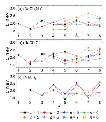
Fig. 4 Dissociation energies of the (a) cations, reaction (2); (b) anions, reaction (3) and (c) neutrals, reaction (4) as a function of cluster size x. Dissociation from the lowest energy isomer of the precursor to the lowest energy isomers of the products is assumed. Calculations are performed at the CCSD/DZ//B3LYP-D3 level
