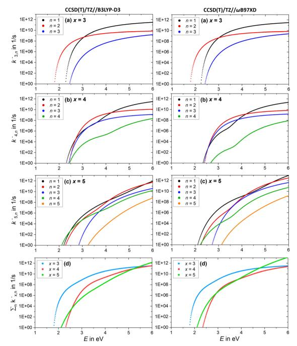
Fig. 9 (a)–(c) Calculated RRKM rate constants  $k_{x,n}^-$  for the loss channels (3) of the precursor ions (NaCl)<sub>x</sub>Cl<sup>-</sup> with x = 3-5. Note that the loss channels producing  $Cl^-$  ions  $(k_{x,n=x}^-)$  are always the slowest. (d) Total fragmentation rate constants  $\sum k_{x,n}^-$  as sum of all loss channels n for cluster sizes x=3-5.
