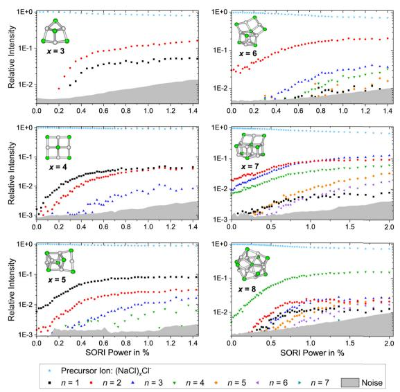
SORI CID spectra of the sodium chloride cluster ions (NaCl)<sub>x</sub>Cl<sup>-</sup> with x = 3-8. The stoichiometric loss channels (3) are observed
