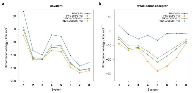
Fig. 4 Comparison of computed dimerization energies using different methods and the awcvgz basis (see text) for the (a) covalent and (b) weak donoracceptor bound systems depicted in Fig. 3.
