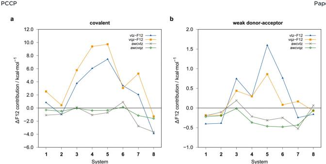
Fig. 7  $\Delta F_{12} = \Delta E_{\text{LMP2-F12(PAO)}} - \Delta E_{\text{LMP2}}$  contributions in to the binding energies (THRPNO\_LMP2=1d-10) in kcal mol<sup>-1</sup>. (a) Covalent dimers, (b) weak donor-acceptor dimers. vgz-f12 values computed with  $\gamma$  (opt3), otherwise  $\gamma$  = [1.0,1.4] was employed.
