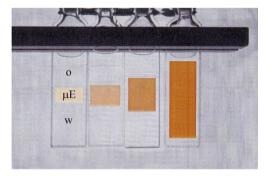
Fig. 6 Illustration of the growth of the middle phase of the Winsor III system based on decane-water- $C_{12}E_4$  with different amounts of the amphiphilic polymer PEP-PEO added. The surfactant + polymer content was kept constant, 3 weight%, and the ratio polymer/polymer + surfactant increased from left to right: 0; 0.015; 0.050; 0.115. (Reproduced from ref. 27 with permission from the American Chemical Society, copyright 1999.)
