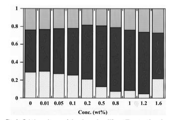
Fig. 4 Relative volumes of the phases in a Winsor III system based on decane, water and C<sub>12</sub>E<sub>5</sub> as a function of added HM-EHEC. All vials are composed of an upper phase (grey), a middle phase (black) and a lower phase (white). (Reproduced from ref. 26 with permission from the American Chemical Society, copyright 1994.)
