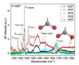
Fig. 19 Sum frequency spectra of a 24 h stearic acid-modified calcite surface in the double-bond/fingerprint region collected under the SSP, PPP, SPS, SSS, and SPP polarization combinations at  $\Psi$  = 240°. Proposed assignments and sketches of the carboxylic and carboxylate groups are included in the figure. Figures reproduced from Wojas et al., Langmuir., 2023, **39**, 14840. 122
