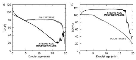
Fig. 21 Contact angle (a) and droplet base diameter change (b) on stearic acid-modified calcite and polystyrene. The data becomes scattered when the droplet becomes very small, as seen after about 17 minutes. Figures adopted from Wojas et al., Langmuir., 2021, 37, 14135. 129
