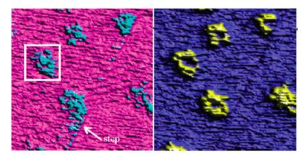
Fig. 8 Height (left) and surface potential (right) on a calcite surface with hillocks at a RH level of 45% measured using Kelvin probe force microscopy. The image size is  $3 \times 3 \, \mu m^2$ . The surface potential difference between the hillocks and the terrace is about 120 mV, with the former displaying the less negative values. Reprinted with permission from Na *et al.*, *Environ. Sci. Technol.*, **41**, 6491. Copyright 2007 American Chemical Society.<sup>74</sup>
