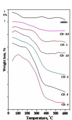
**Fig. 16** TGA curves for calcite modified by stearic acid. The data is shown for calcite powder and samples with different degree of coverage given within brackets. CD-0.5 (0.52), CD-1 (1.00), CD-1.5 (1.53), CD-2 (2.16), CD-3 (3.25), CD-4 (4.44). Figure reproduced with permission from Mihajlovic *et al.*, *Powder Technol.*, 2013, **245**, 208. Copyright 2013 Elsevier.<sup>123</sup>
