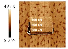
Fig. 10 An image of the tip-sample adhesion after wear measurements in dry (<5% RH) air. The redeposited hillocks are completely removed from the worn area. The image size is  $2 \times 2 \mu m^2$ . Figure from Wojas et al., Langmuir., 2021, 37, 9826.79
