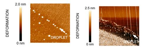
Fig. 20 AFM deformation images of the region close to the water droplet edge, imaged in air after removal of the droplet. Left: Octanoic acid-coated calcite, image size  $10 \times 10 \ \mu m^2$ . Right: Stearic acid-coated calcite, image size  $40 \times 40 \ \mu m^2$ . The position of the three-phase line is indicated by the white arrow, and the droplet covered the lower left side of the image. Figures reproduced from Wojas et al., Langmuir., 2021, **37**, 14135. 129
