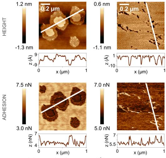
Fig. 17 AFM images of topography (top) and adhesion (bottom) showing the calcite (10 14) surface plane after exposure to stearic acid vapour for 20 min at 85 °C (left) and 105 °C (right). Line profiles along the white lines are shown below each image. Figures reproduced from Wojas et al., Langmuir., 2023, **39**. 14840. 122
