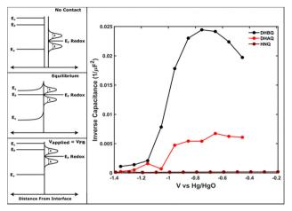
Fig. 3 Semiconducting electrode-electrolyte interface, and the basis for the Mott-Schottky analysis (exaggerated for clarity). Upon contact, the semiconductor and electrolyte equilibrate in electron energies, and at the flat band potential ( $V_{\rm FB}$ ) the solid returns to the equilibrium (bulk) band structure. This flat band potential ( $V_{FB}$ ) is quantitatively the x-intercept of the inverse capacitance with applied bias.
