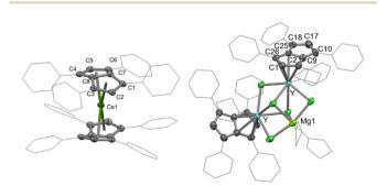
Fig. 3 Molecular structures of (left) the anion of 1-Ce(DME) and (right) the anionic MgY<sub>2</sub> pentalenide cluster of 3. Selected ellipsoids drawn at 50% probability; H atoms, counter cations and lattice solvent omitted for clarity.
