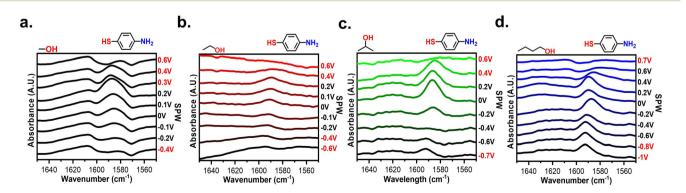
Fig. 7 Spectra of a 4-MA modified SEIRAS substrate at different applied potentials within 0.1 M LiCl (a) MeOH, (b) EtOH (c) IPA, and (d) BuOH. The voltages marked in red denote applied potentials beyond the CV-based SPW.
