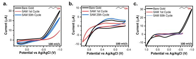
Fig. 5 Comparing a baseline CV in 0.1 M LiCl BuOH against a 4-MA covered electrode when (a) cycled negatively beyond the SPW and (b) when cycled positively beyond SPW. (c) A scheme of the SPW of thiolate SAMs in non-aqueous solvents.
