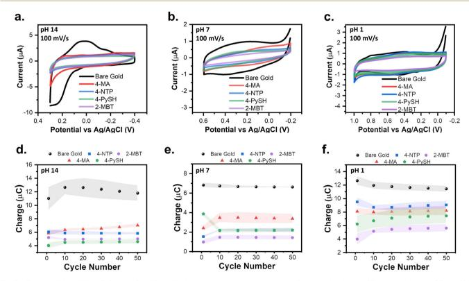
Fig. 3 CVs of 4-MA, 4-NTP, 4-PySH, and 2-MBT modified electrodes compared to baseline CVs cycled within the SPWs established for (a) 1 M KOH (pH 14), (b) 0.1 M NaCl (pH 7), and (c) 0.1 M HClO<sub>4</sub> (pH 1). The average integrated charge from the anodic sweeps of the baseline and modified electrodes CVs plotted *versus* the cycle number in (d) KOH, (e) NaCl, and (f) HClO<sub>4</sub>. The shaded regions depict the standard deviation of each measurement for three independent measurements.
