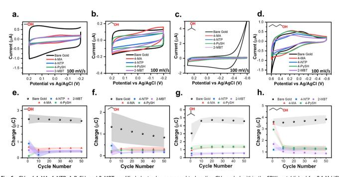
Fig. 6 CVs of 4-MA, 4-NTP, 4-PySH, and 2-MBT modified electrodes compared to baseline CVs cycled within the SPWs established for 0.1 M LiCl (a) MeOH, (b) EtOH, (c) IPA, and (d) BuOH. The average integrated charge from the anodic sweeps of the baseline and modified electrodes CVs plotted versus the cycle number in (e) MeOH, (f) EtOH, (g) IPA, and (h) BuOH. The shaded regions depict the standard deviation of each measurement for three independent measurements.
