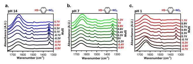
Fig. 4 Spectra of a 4-NTP modified gold-plated IRE at different applied potentials within (a) 1 M KOH (pH: 14), (b) 0.1 M NaCl (pH: 7), and (c) 0.1 M HClO<sub>4</sub> (pH: 1). The potentials marked in red denote those beyond the CV-based SPW.
