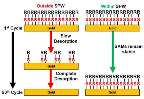
Scheme 2 Depiction of slow desorption of thiolate SAMs on gold in non-aqueous solvents when cycling to potentials outside the SPW and the retention of the SAM when cycled within the SPW.
