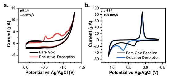
Fig. 1 CVs in degassed 1 M KOH showing the (a) reductive desorption and (b) oxidative desorption of 4-PySH compared to baseline bare gold CVs.
