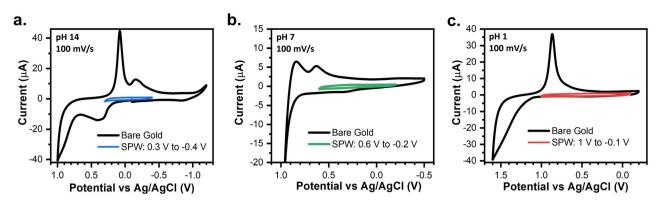
Fig. 2 CVs of a bare gold electrode compared to a 4-PySH-covered electrode cycled within the SPW in (a) 1 M KOH (pH 14), (b) 0.1 M NaCl (pH 7), and (c) 0.1 M HClO<sub>4</sub> (pH 1).
