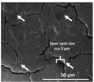
Fig. 2 SEM characterization of ultrathin Ag film (6 nm) deposited using thermal evaporation. Off-tissue image of an ITO glass slide at 120 000× magnification (left). On-tissue image at 800x magnification showing the laser spot size (right).
