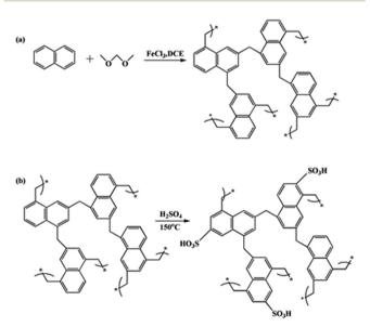
Scheme 1 The structures of the polymer and solid acid. (a) POP-0.01, (b) POP-0.01-SO<sub>3</sub>H-30.
