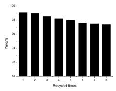
The reuse of POP-0.01-SO<sub>3</sub>H-30 for biodiesel sythesis.
