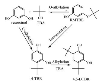
Scheme 3 The possible reaction mechanism for t-butylation.
