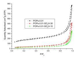
Fig. 7 Nitrogen adsorption-desorption isotherms
