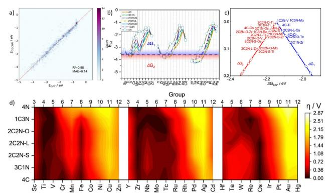
Fig. 10 Taken from Fig. 3 and 4 in Lian et al.<sup>211</sup> (a) DFT calculated and machine learning predicted adsorption energy of Li-polysulfides, (b) predicted adsorption energy of LiS\*, (c) volcano plots for catalysts with an overpotential lower than 0.1 V, and (d) heat map of the predicted overpotential of different SACs. Reproduced with permission.<sup>211</sup> Reprinted (adapted) with permission from ref. 211. Copyright 2021 American Chemical Society.
