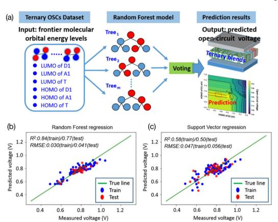
Fig. 4 (a) Using the values of the HOMO and LUMO as features in the ternary OPV  $V_{\rm OC}$  prediction model. (b) The RF model and (c) SVM model. (6) Reproduced from ref. 69 under the terms of the Creative Commons Attribution License from Wiley.
