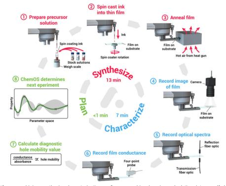
Fig. 9 8-Step auto-platform combining synthesis, characterization, software machine learning calculation into a self-driving workflow to make thin film samples, this work reported by Macleod et al. 176 Reproduced from ref. 176 under a Creative Commons Attribution NonCommercial License 4.0 (CC BY-NC).
