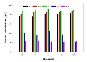
Fig. 3 The photocatalytic activity of paints P-1, P-2, P-3, P-4, and P-5 against 3 ppm toluene with a total flow rate of 50 mL min<sup>-1</sup>, under 24 W white light.
