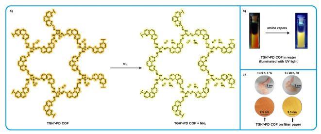
Fig. 7 TGH+-PD based "turn-on" fluorometric amine sensor. (a) Mechanism for the interaction of TGH+-PD with ammonia. (b) Modified images showing the resulting change in photoluminescence of TGH+.PD water dispersions from Trabolsi et al. (c) Modified images showing the color of TGH+.PD on filter paper after exposure to fresh and rotting chicken wit permission from Trabolsi et al. 127
