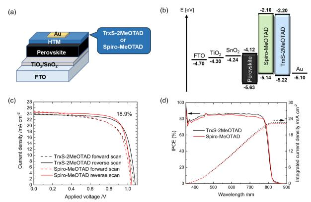
Fig. 7 (a) The PSC device structure employed in this study. (b) The corresponding energy level diagram. The values for FTO,  $TiO_2$ ,  $SnO_2$  and Au were taken from the literature. (c) J-V curves of the best TrxS-2MeOTAD PSC and spiro-MeOTAD PSC fabricated in this study. (d) The corresponding IPCE curves.
