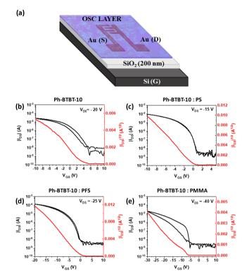
Fig. 3 (a) Schematic illustration of the OFET architecture. Transfer characteristics in the saturation regime of the OFETs based on Ph-BTBT-10 (b), and Ph-BTBT-10 blended with PS (c), PFS (d) and PMMA (e).
