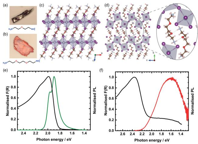
Fig. 1 (a) OBESnI<sub>4</sub> and (b) EDBESnI<sub>4</sub> images of mm-sized single crystals. Crystal structure of (c) OBESnI<sub>4</sub> and (d) EDBESnI<sub>4</sub>, where grey atoms are Sn, purple are I, blue are N, brown are C, red are O, and white are H. The inset highlights the formed hydrogen bonds. Kubelka-Munk transformed diffuse reflectance and photoluminescence spectra of (e) OBESnl<sub>4</sub> and (f) EDBESnl<sub>4</sub>
