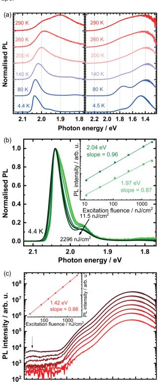
Fig. 2 (a) Temperature-dependent photoluminescence spectra of OBESnl<sub>4</sub> (left panel) and EDBESnI<sub>4</sub> (right panel). Power-dependent photoluminescence spectra at 4.4 K of (b)  $OBESnI_4$  and (c)  $EDBESnI_4$ , where the insets show the doublelogarithmic plots of the photoluminescence intensity versus excitation fluence.
