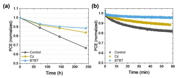
Fig. 5 Stability test on PSCs without encapsulation in (a) ambient conditions (25% RH) and (b) under continuous illumination and MPPT conditions.
