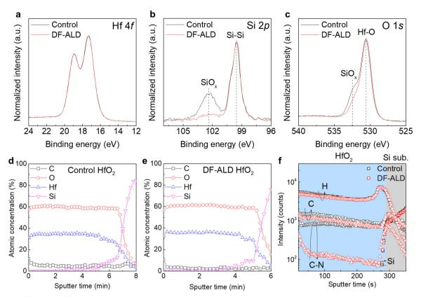
Fig. 2 (a) Hf 4f, (b) Si 2p, and (c) and O 1s core level XPS spectra of HfO<sub>2</sub> films grown via the control and DF-ALD processes. AES depth profiles of Hf, O, Si, C and N of the (d) control and (e) DF-ALD HfO2 films. (f) ToF-SIMS depth profiles of H, C and C-N in the control HfO2 and DF-ALD HfO2 thin films.
