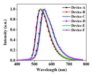
Fig. 4 Electroluminescence (EL) curves at 5 V for PSeDBF and PSeFL devices
