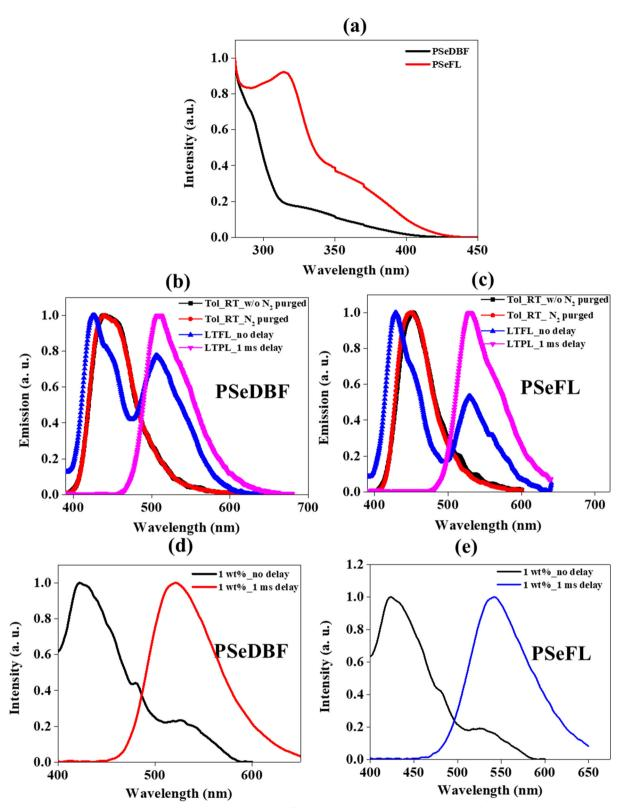
Fig. 3 (a) UV-Visible curves of PSeDBF and PSeFL measured using  $10^{-5}$  M toluene solution. PL measured in  $10^{-5}$  M toluene solution without and with nitrogen bubbling at room temperature and low-temperature PL in  $10^{-5}$  M toluene solution without (LTFL) and with 1.0 ms delay (LTPL) for (b) PSeDBF and (c) PSeFL. PL measured using 1 wt% emitters dopped in mCP-TSPO1 host film at room temperature without and with 1.0 ms delay for (d) PSeDBF and (e) PSeFL.
