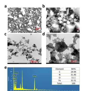
Fig. 2 (a) and (b) FE-SEM images, (c) and (d) HR-TEM images, and (e) EDS spectra of FeNP (inset table shows the elemental wt%).
