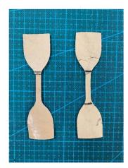
Fig. 33 Dumbbell test piece of (Left) natural rubber and (Right) natural rubber nano cellulose composite material. 180
