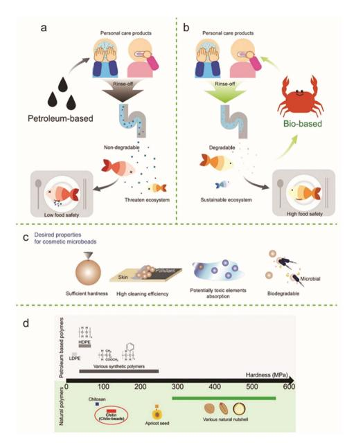
Fig. 36 Applications of microbeads in daily care products and their potential impacts on the environment. (a) Petroleum-based microplastics and their main risks. (b) Bio-based microplastics and their desired consequences for sustainable cosmetics. (c) Desired cosmetic microbead properties and (d) comparison of the hardness between the materials in this study and some natural and synthetic abrasive materials (HDPE: high-density polyethylene and LDPE: low-density polyethylene).<sup>166</sup>
