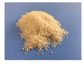
Fig. 10 PLA-based 100% biomass biodegradable plastic for injection, biaxial stretch blow molding.<sup>59</sup>
