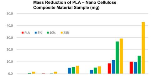
Fig. 4 Biodegradability test result. It can be seen that biodegradability increased as the content of nanocellulose increases in the PLA-nano-cellulose composite material.<sup>49</sup>
