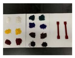
Fig. 23 Biomass biodegradable color masterbatch.
