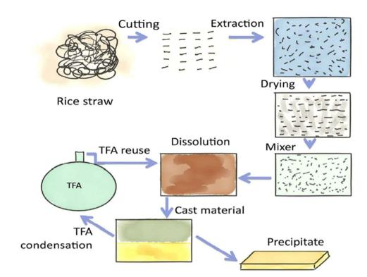
Fig. 41 Synthesis of bioplastics from rice straw (TFA: trifluoroacetic acid). 180
