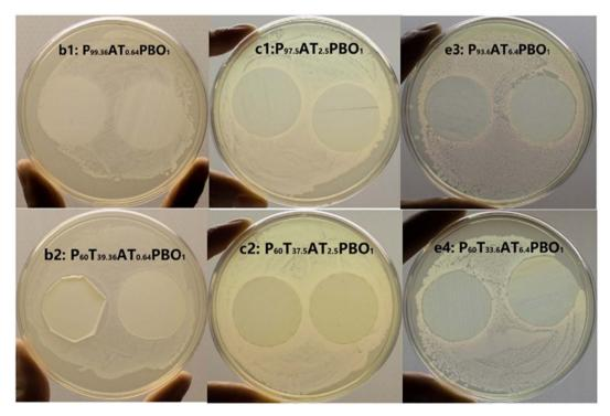
Fig. 34 Pictures of different anti-bacterial PBAT films against *Escherichia coli* tested using the ring diffusion method. The subscripts represent the contents of the compositions. Where, P: PBAT, T: TPS (thermoplastic starch), AT: ATPS (anti-bacterial thermoplastic starch), and PB: 2,2'-(1,3-phenylene)-bis (2-oxazoline) as the coupling agent.<sup>164</sup>
