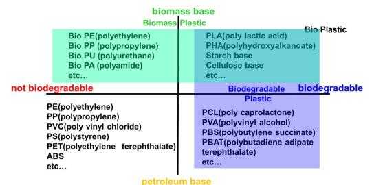
Fig. 2 Classification of plastic according to biomass and biodegradability
