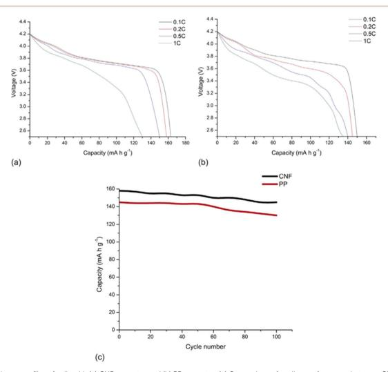
Fig. 14 Discharge profiles of cells with (a) CNF separator and (b) PP separator. (c) Comparison of cycling performance between CNF separator and PP separator.<sup>80</sup>
