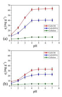
Fig. 15 Adsorption efficiencies of extracted cellulose, cell-EDTA (ethylene diamine tetra acetic acid-modified nanocellulose), and cell-CM (carboxy methyl group-modified nanocellulose) for (a) Pb2+ and (b) Cd<sup>2+</sup> in the pH range of 1–7. Conditions for adsorption: concentration of  $Pb^{2+}$  or  $Cd^{2+} = 100 \text{ mg L}^{-1}$ , at room temperature for 90 min.81
