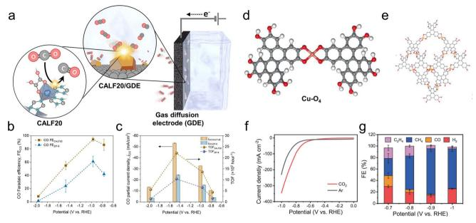
Fig. 6 Zn-based CALF20 features ligand-based active sites (a) whose electron-rich structure facilitates  $CO_2R$  to CO more than a ZIF-8 analogue (b and c). <sup>87</sup> Cu- $O_4$  active sites (d) within a Cu-BTC MOF (e) exhibit both high activity (f) and selectivity (g) for  $CO_2R$  to  $CH_4$ . <sup>95</sup> Reproduced with permission from the American Chemical Society, copyright 2021 and Springer Nature, copyright 2021.
