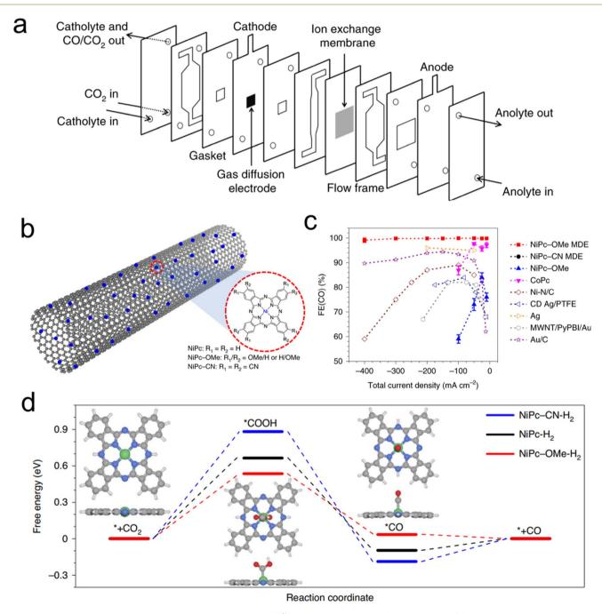
Fig. 4 The typical electrolyser configuration employing GDEs (a),  $^{61}$  a scheme of catalyst-CNT integration (b), effects of functional groups on performance (c), and free-energy landscape of CO<sub>2</sub>R (d),  $^{46}$  reproduced with permission from Springer Nature copyright 2019.
