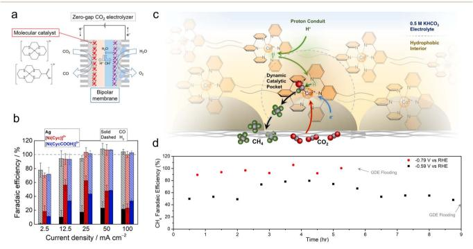
Fig. 5 Ni cyclam catalysts were integrated with bipolar membrane electrolysers (a), in which they reduced  $CO_2$  to CO (b).<sup>74</sup> Proton shuttling enables  $CO_2R$  within a hydrophobic pocket within GDE electrodes (c) and shifts the reaction selectivity to  $CH_4$ , with a selectivity of almost unity (d).<sup>78</sup> Reproduced with permission from the American Chemical Society, copyright 2022.
