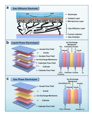
Fig. 2 (a) Schematic diagram of a gas diffusion electrode. (b) Schematic diagram and cross-sectional view of a liquid phase electrolyser. (c) Schematic diagram and cross-sectional view of a gas phase electrolyser. Reproduced from ref. 36. Copyright 2021 Wiley-VCH.
