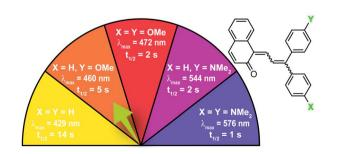
Fig. 6 Electron-donating para-substituents result in bathochromically shifted (longer wavelength) merocyanine absorption and increase the rate of thermal reversion. Values shown were measured in toluene at 20  $^{\circ}$ C.  $^{37}$
