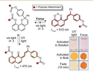
Fig. 11 In contrast to the reversible photochemical reaction, mechanochemical activation of a 2H-naphthopyran mechanophore with polymer attachment via an ester linkage at the 10-position generates a persistent merocyanine dye stabilized by an intramolecular hydrogen bonding interaction that is established upon scission of the C(O)-O ester bond
