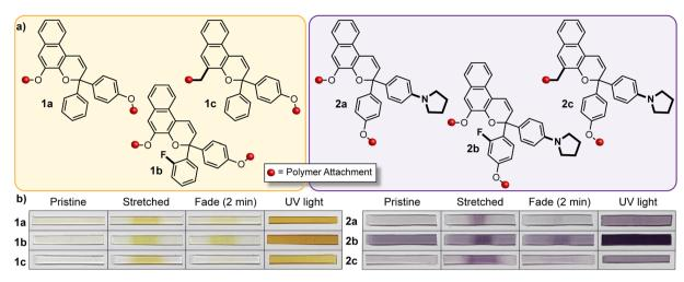
Fig. 9 (a) Different 3*H*-naphthopyran mechanophores with varying substitution affecting merocyanine color and reversion rate. (b) Photographs of polydimethylsiloxane samples covalently incorporating the naphthopyran crosslinkers before and after being subjected to uniaxial tension and subsequent stress relaxation, or UV light irradiation, demonstrating the modularity of the naphthopyran mechanophore for designing mechanochromic materials. Adapted from ref. 145.
