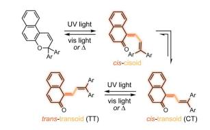
Scheme 10 Exemplary photochemical ring-opening reaction of a 3*H*-naphthopyran and alkene isomerization to generate principal *cis*-transoid (CT) and *trans*-transoid (TT) isomeric merocyanine products.
