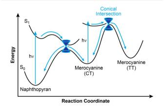
Fig. 3 Representative reaction pathway for the photochemical ringopening reaction of naphthopyran.
