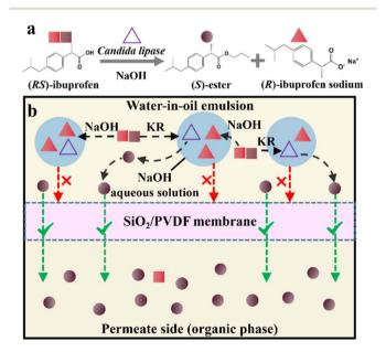
Fig. 31 (a) Coupled strategy of membrane-enhanced enzymatic kinetic resolution by Candida lipase and (b) schematic representation of gravity-driven penetration of the reaction mixture through SiO<sub>2</sub>/ PVDF membranes.340
