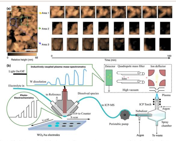
Fig. 6 (a) In situ EC-AFM images of the  $BiVO_4$  photoanode. Three coloured boxes represent area 1 (yellow), area 2 (green) and area 3 (blue), of which operando scans are recorded in detail. Reprinted with permission from ref. 67, copyright 2016, Nature Publishing Group. (b) Schematic combination of the inductively coupled plasma mass spectrometry (ICP-MS) and the illuminated scan flow cell (SFC). Reprinted with permission from ref. 71, copyright 2018 Elsevier B.V.
