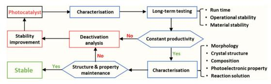
Fig. 2 Proposed stability assessment process of photocatalysts/photoelectrodes for solar fuel production.
