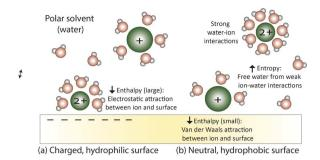
Fig. 6 Average surface interactions at (a) a charged, hydrophilic surface where electrostatic forces dominate and attract small, strongly hydrated ions and (b) a neutral, hydrophobic surface where hydrophobic forces, a combination of entropic forces and van der Waals interactions, dominate to stabilize large, weakly hydrated ions at the surface.
