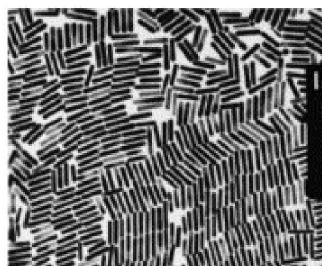
Fig. 4 (a) Shows a schematic diagram of the setup for (GNR) electrochemical preparation and (b) shows (TEM) images of (GNR) with various aspect ratios. They are reprinted with permission from ref. 100 © 1999 American Chemical Society.
