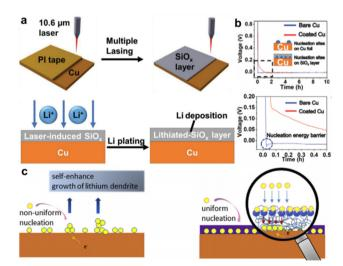
Fig. 3 Non-metal lithiophilic sites. (a) Schematic diagram for the formation of laser induced  $SiO_x$  layer on the Cu CC and the lithium plating behavior. (b) Voltage profile of bare Cu and Cu with LI-SiO<sub>x</sub> layer. Reproduced with permission.<sup>37</sup> Copyright 2020 Wiley-VCH Verlag GmbH & Co. KGaA, Weinheim. (c) Schematic of the mechanism of PDA-induced Li deposition. Reproduced with permission.<sup>39</sup> Copyright 2019 Elsevier B.V.
