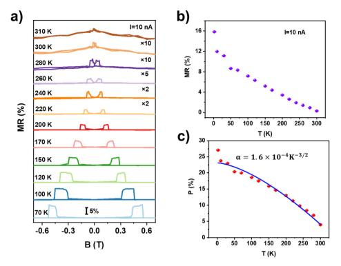
Fig. 5 Temperature-dependence of the spin-valve effect in the Fe<sub>3</sub>GaTe<sub>2</sub>/MoS<sub>2</sub>/Fe<sub>3</sub>GaTe<sub>2</sub> device. (a) MR curves measured at different temperatures from 70 K to 310 K with a fixed bias current of 10 nA. (b) The extracted MR ratios as a function of temperature. (c) Spin polarization as a function of temperature. The blue line is the fitting curve according to the Bloch law.
