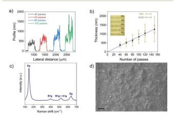
Fig. 2 (a) Surface profiles of inkjet-printed TiO<sub>2</sub>-NS lines on the glass substrate measured by profilometry. (b) Average thickness of the printed TiO<sub>2</sub>-NS lines on glass substrate plotted as a function of the number of passes. RMS = root mean square, STDEV = standard deviation. (c) Raman spectrum of the TiO<sub>2</sub>-NS film printed on the glass substrate. (d) Topview SEM image of a printed film dried at 45 °C (platen temperature), scale bar =  $2 \mu m$ .
