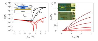
Fig. 5 (a) Channel current (black curve) and gate current (red curve) as a function of  $V_{\rm GS}$  with  $V_{\rm DS}$  = 2 V. In the inset, a sketch of the longitudinal section of the structure, showing its layer sequence and biasing voltages. (b) Output characteristics measured for  $V_{GS}$  ranging from -1 to 3 V, with a step of 0.5 V. The inset shows optical micrographs of a device before and after TiO<sub>2</sub> printing. The scale bars are 100 um.
