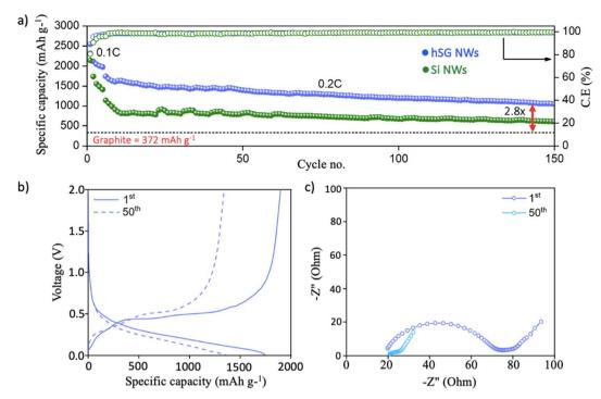
Fig. 3 (a) Cyclic performance of hSG NWs and Si NWs at 0.2C cycled between 0.011-2.0 V, (b) corresponding voltage-specific capacity plot and (c) EIS analysis of hSG NWs after  $1^{\text{st}}$  and  $50^{\text{th}}$  cycle of hSG NWs.
