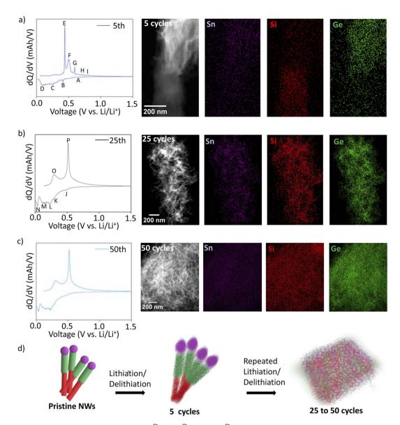
Fig. 4 Differential capacity plot of hSG NWs after (a) 5<sup>th</sup>, (b) 25<sup>th</sup> and (c) 50<sup>th</sup> cycle at 0.2C with corresponding STEM and EDX images. (d) Schematic illustration of the structural evolution of hSG NW during Li cycling.
