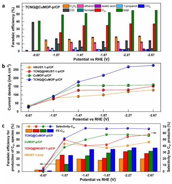
Fig. 4 (a) Catalytic performance of the TCNQ@CuMOP-p/CP electrode for CO<sub>2</sub>RR at different potentials. (b) Comparation of the total current density over different electrodes for CO<sub>2</sub>RR at different potentials. (c) Faradaic efficiency (FE) and selectivity to C<sub>2+</sub> products over different electrodes for CO<sub>2</sub>RR at different potentials.
