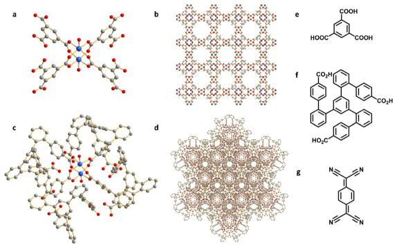
Fig. 1 Views of (a) the  $[Cu_2(OOCR)_4]$  paddlewheel in HKUST-1; (b) structure of HKUST-1; (c) the  $[Cu_2(OOCR)_4]$  paddlewheel in CuMOP; (d) structure of CuMOP; (e) benzene-1,3,5-tricaroxylic acid used in HKUST-1; (f) ligand used in CuMOP; (g) TCNQ. Cu: blue; O: red; C: grey; hydrogen atoms are omitted for clarity.
