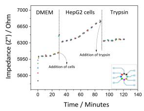
Fig. 8 Impedance recording of HepG2 cell culture measured at 100 Hz showing cell adhesion and detachment (short-term measurements lasting for 2 hours). Each color represents a different electrode.
