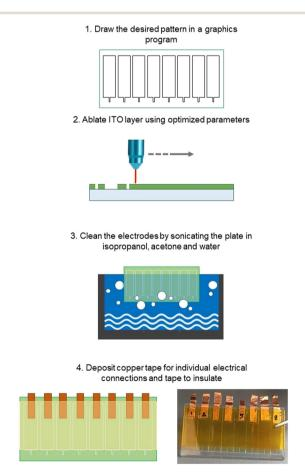
Fig. 1 Step-by-step fabrication procedure of the directly ablated patterns
