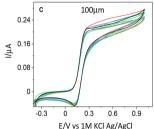
Fig. 5 Cyclic voltammograms of electrodes of different sizes (a) 25, (b) 50 and (c) 100  $\mu$ m width, 2.5 mm length in 1 mM FcDM and 0.1 M KNO $_3$  at 100 mV s $^{-1}$ . Each set of electrodes comes from the same plate.
