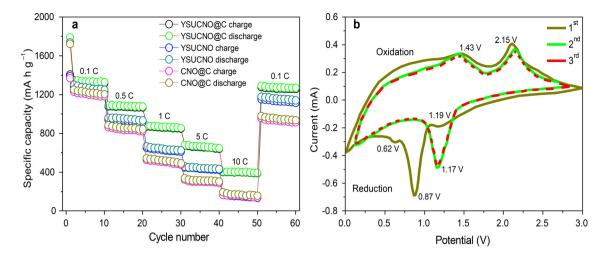
Fig. 4 (a) Rate performance of the YSUCNO, YSUCNO, and CNO microspheres and (b) the cyclic voltammetry curves of the first three cycles of the YSUCNO, microspheres.
