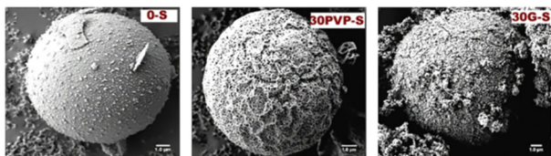
Fig. 3 SEM images of NaAlO 2 catalysts prepared through a spray-drying (S) method without an organic template (left) or with the addition of polyvinylpyrrolidone (PVP, centre) or glycerol (G, right) as a template. Reproduced from "Production of Glycerol Carbonate from Glycerol over Templated-Sodium-Aluminate Catalysts Prepared Using a Spray-Drying Method" P. Rittiron, C. Niamnuy, W. Donphai, M. Chareonpanich and A. Seubsai, ACS Omega , 2019, 4, 9001–9009 (ref. 91), https://pubs.acs.org/doi/10.1021/acsomega.9b00805 .
