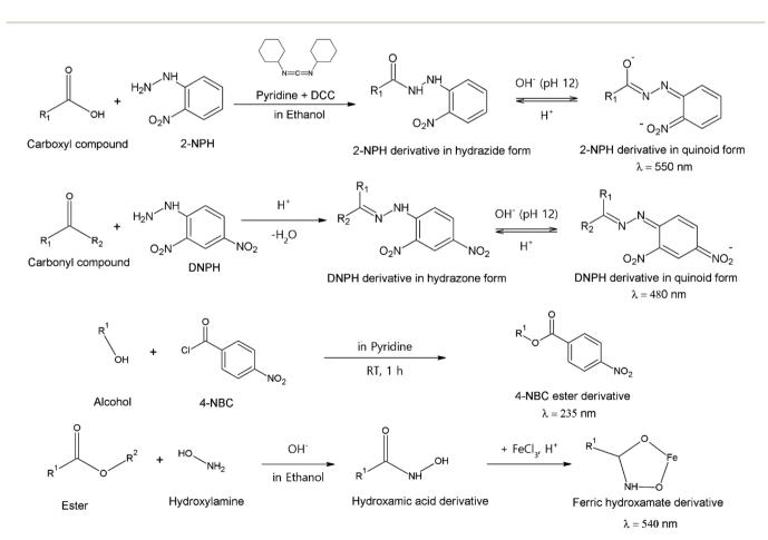
Fig. 3 Functional group-specific reactions and measurement wavelengths ( $\lambda$ ) applied in spectrophotometric application. Reproduced from ref. 108 with permission from Taylor & Francis Group, copyright 2013.
