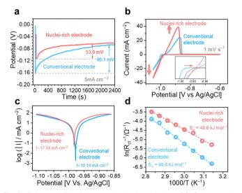
**Fig. 4** Enhanced Zn plating and stripping kinetics. (a) Galvanostatic voltage profiles, (b) cyclic voltammograms curves, (c) Tafel plots, and (d) Arrhenius plots of Zn plating and stripping on conventional and nuclei-rich electrodes.
