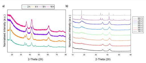
Fig. 12 (a) PXRD of Li<sub>2</sub>SnO<sub>3</sub> with increasing mill time. Conversion to DRS occurs at ~8 h (b) Plot showing the changes in PXRD pattern with increasing temperature, showing the transformation from DRS to layered on heating. (Cu Ka).
