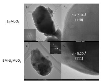
Fig. 4 TEM images of pristine (a) and ball milled (c) Li<sub>2</sub>MoO<sub>4</sub> particles, with inset images showing the SAD pattern recorded on the particles, and the respective HR-TEM images (b and d) clearly showing the lattice fringes. The observed interplanar distance from the fringes have been indexed.
