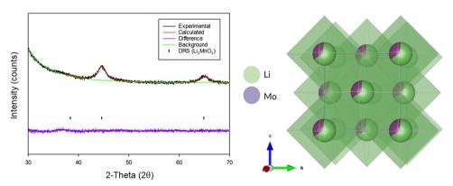
Fig. 10 Observed, calculated and difference plot from the Rietveld refinement of BM-Li<sub>2</sub>MnO<sub>3</sub> after 16 h (Cu Kα) and an image of the crystal structure.
