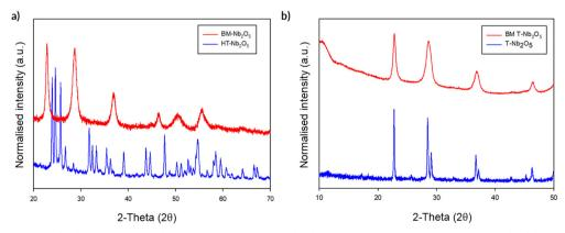
Fig. 14 (a) High temperature (HT) phase – H-Nb<sub>2</sub>O<sub>5</sub> before and after milling (BM) showing a phase conversion to T-Nb<sub>2</sub>O<sub>5</sub>. (b) Low temperature phase (T-Nb<sub>2</sub>O<sub>5</sub>) before and after milling showing no change in structure, just broadening of the peaks due to the smaller particle size after milling. (Cu Kα).
