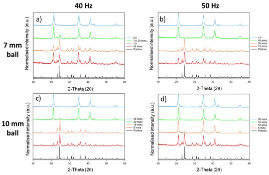
Fig. 6 Resulting PXRD patterns from the study of ball mill frequency, time and ball size on the milling of Li<sub>2</sub>MoO<sub>4</sub>. Patterns (a) and (b) made use of a 7 mm ball at 40 Hz and 50 Hz, respectively. Patterns (c) and (d) made use of a 10 mm ball at 40 Hz and 50 Hz respectively. The conversion rate was shown to significantly reduce with lower frequency or ball size. (Co  $K\alpha$ ). 50 mg of material was loaded into the pots in each case.
