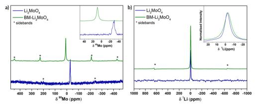
Fig. 3 (a)  $^{95}$ Mo NMR for Li<sub>2</sub>MoO<sub>4</sub> and BM-Li<sub>2</sub>MoO<sub>4</sub> at 700 MHz (16.4 Tesla), 10 kHz MAS, single pulse spectra. (b)  $^{7}$ Li NMR at 200 MHz (4.7 Tesla), 50 kHz MAS, with 1  $\mu$ s pulse for Li<sub>2</sub>MoO<sub>4</sub> and BM-Li<sub>2</sub>MoO<sub>4</sub>. In both figures, inset focuses on the central transition peak.
