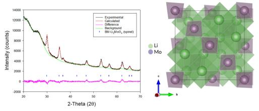
Fig. 2 Observed, calculated and difference profiles for Rietveld refinement of BM-Li<sub>2</sub>MoO<sub>4</sub> (16 h) (left) and an image of the spinel structure adopted by this phase (right). (Cu  $K\alpha$ ).
