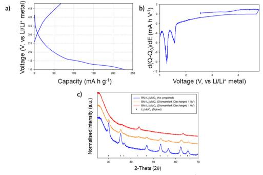
Fig. 7 (a) First cycle voltage profile for BM-Li<sub>2</sub>MoO<sub>4</sub> cycled in the region of 4.8-1.0 V at 10 mA  $g^{-1}$ ; (b) associated dQ/dV plot of the first charge/ discharge cycle; (c) PXRD of dismantled swagelok cells showing phases formed once discharged down to 1.5 and 1.0 V (Cu Kα).
