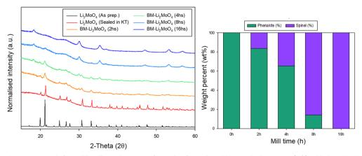
Fig. 1 PXRD of samples prior to and after milling illustrating a transformation from phenakite to spinel structure (left), with the calculated phase fractions from Rietveld refinement (right). (Cu Kα). Note: the high background in samples after milling can be attributed to the Kapton tape (KT) used to measure the material to prevent air exposure
