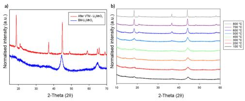
Fig. 11 (a) PXRD of BM-Li<sub>2</sub>MnO<sub>3</sub> sample before (DRS phase) and after VT-PXRD (layered phase) (b) VT-PXRD experiment in the region of 100–800 °C showing the change in the relative intensity of peaks with increasing temperature indicating a transformation from DRS to layered on heating. (Cu Kα).
