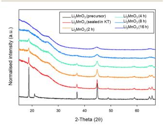
Fig. 9 PXRD data for the timed milling study of  $Li_2MnO_3$  (2–16 h at 450 rpm) showing a transition from a layered to DRS structure (Cu  $K\alpha$ ).
