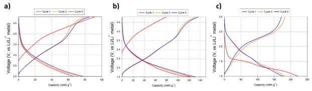
Fig. 8 Voltage profiles for BM-Li<sub>2</sub>MoO<sub>4</sub> using varying voltage ranges: (a) 4.8-2.0 V, (b) 4.8-1.5 and (c) 3.0-1.0 V. Note: cell c was discharged first before charging to higher voltages.
