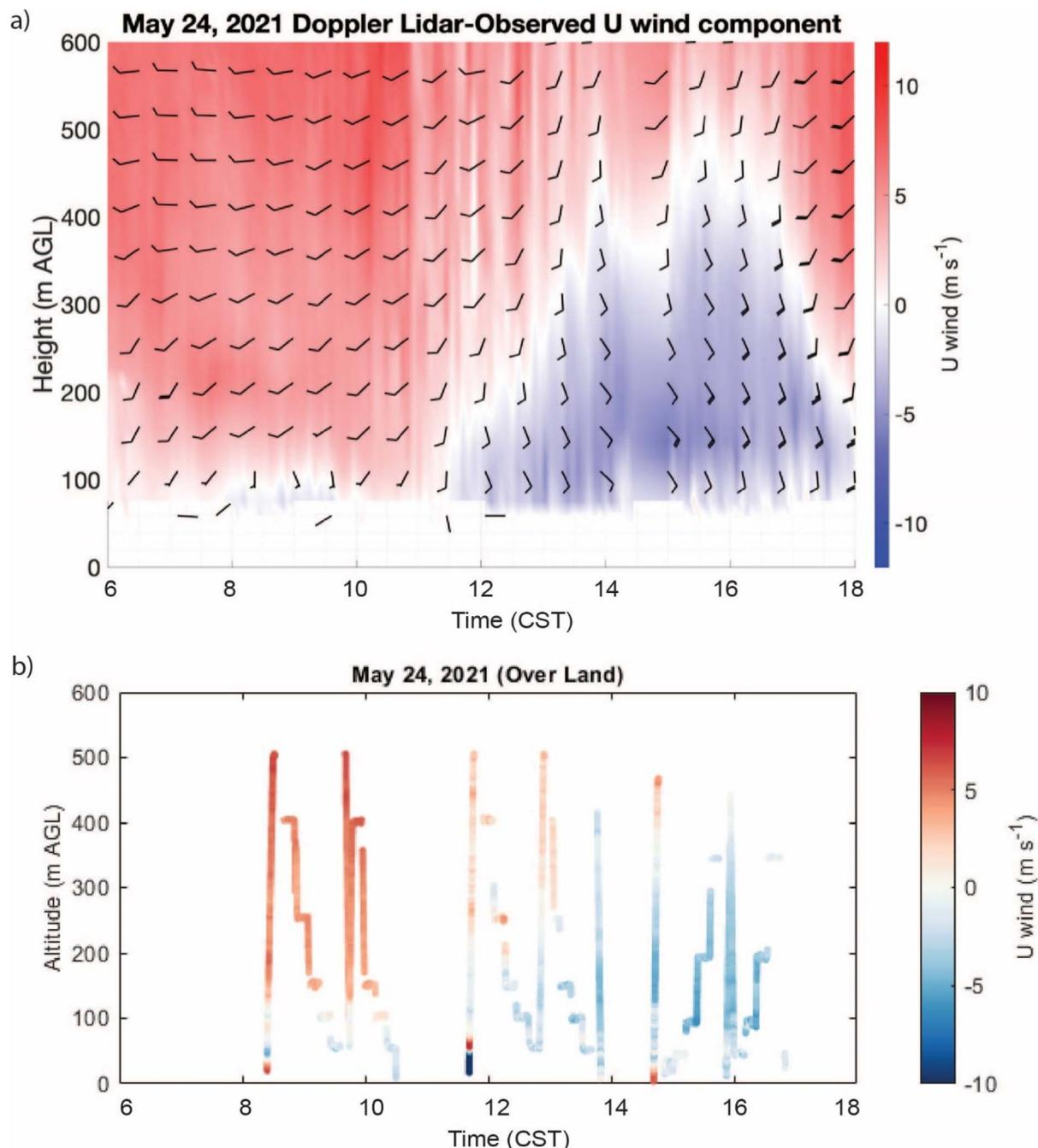
Fig. 5 Time–height cross section of the  $u$  (zonal) wind component from (a) the Doppler-lidar-observed horizontal winds (in  $\text{m s}^{-1}$ ), overlaid with horizontal wind barbs (in knots) plotted from 22 May 2021. Wind barbs are thinned by a factor of 5 in the time dimension and a factor of 2 in the height dimension to aid readability and (b) RAAVEN platform observations collected over land on May 24, 2021.
