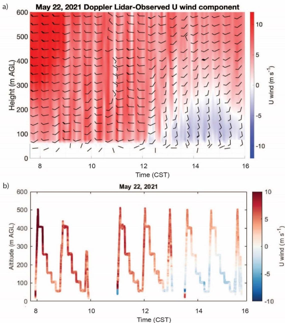
Fig. 4 Time–height cross section of the  $u$  (zonal) wind component from (a) the Doppler-lidar-observed horizontal winds (in  $\text{m s}^{-1}$ ), overlaid with horizontal wind barbs (in knots) plotted from 22 May 2021. Wind barbs are thinned by a factor of 5 in the time dimension and a factor of 2 in the height dimension to aid readability and (b) RAAVEN platform observations collected over land on May 22, 2021. In (a) is reprinted from Earth System Science Data with permission.<sup>32</sup>
