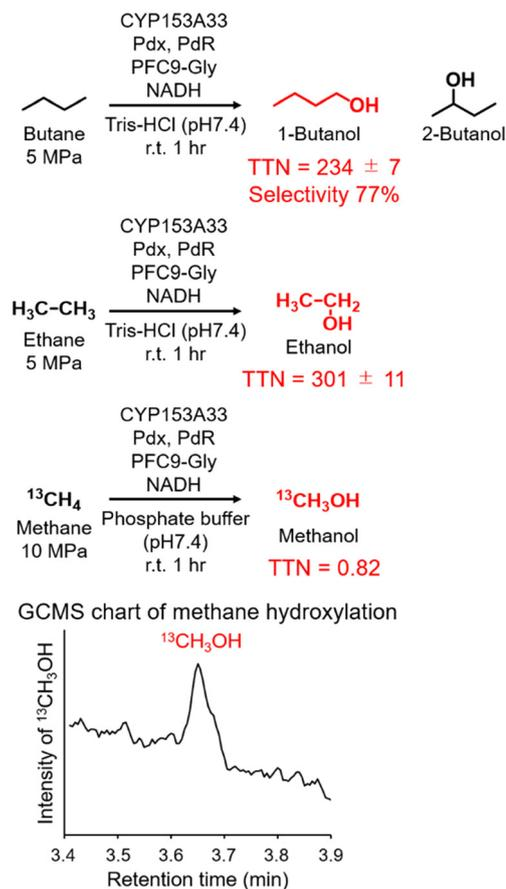
**Fig. 4** Hydroxylation of *n*-butane, ethane, and methane with CYP153A33 in the presence of PFC9-Gly. Reaction conditions: CYP153A33 (1  $\mu$ M), Pdx (10  $\mu$ M), PdR (5  $\mu$ M), substrate gas (*n*-butane and ethane: 5 MPa, methane (<sup>13</sup>CH<sub>4</sub>): 10 MPa), PFC9-Gly (100  $\mu$ M), NADH (5 mM), Tris-HCl buffer (20 mM Tris-HCl, 100 mM KCl, pH 7.4), at room temperature for 1 h.
